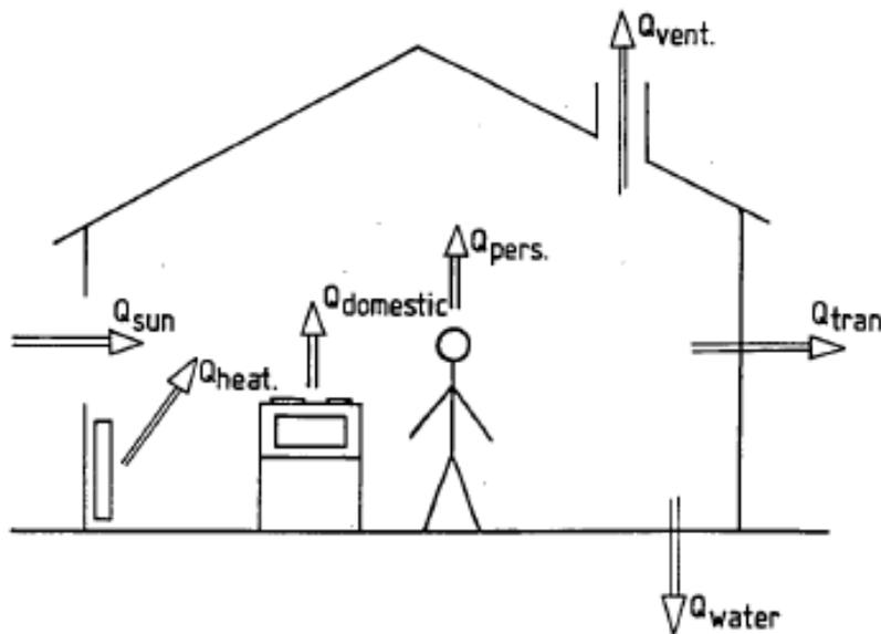
**Figure 2.** Schematic energy balance of a building.<sup>3</sup>
